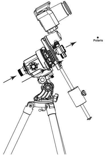
7. Attach **Polar Scope Illuminator** to the dove tail of **Mounting Assembly**. Adjust the position to align it to the **Polar Scope**. This will help make the reticule pattern in the **Polar Scope** eyepiece more visible in dark conditions. Adjust the intensity of the illuminator by turning the dial. Make it bright enough to see the reticule pattern, but not so bright as to wash out your view of Polaris
