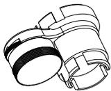
**Polar Scope Illuminator** - To provide lighting source for **Polar Scope**. Also compatible with **Sky-Watcher EQ3, EQ5** and **EQ8**.
