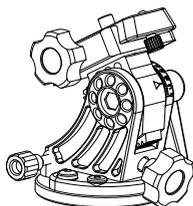
**Equatorial Wedge** - To adjust the latitude of the **Star Adventurer 2i** for polar alignment. Offers higher accuracy and stability than a standard photo tripod head.
