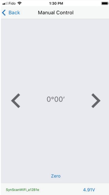
Go to the **Main Menu** and tap on **Manual Control**. This will bring up the manual control arrows on either side of an angle given in degrees and minutes. Tap or touch and hold the arrow symbols to nudge or continuously move **Star Adventurer 2i** to the left or right, respectively. Release the arrow symbol to stop **Star Adventurer 2i**'s movement. The angle you have rotated through will show up between the arrows.
