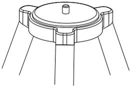
**Without Tilt-head:** take a standard photo tripod or video tripod with a 3/8" connection screw. Spread the legs and secure the tripod legs at the desired height to provide a stable support for your **Star Adventurer 2i**. Assemble **Equatorial Wedge** to the tripod as Fig 1.
