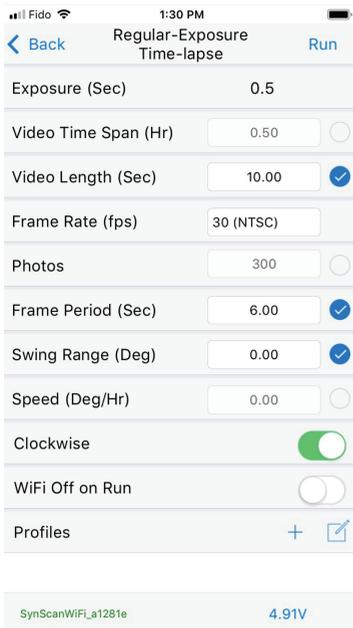
**Exposure (Sec):** Fixed at 0.5 seconds for **Regular-Exposure Time-Lapse**. For **Long-Exposure Time-Lapse** set this value to suit your exposure requirements. Be sure to set your camera shutter to BULB mode.
