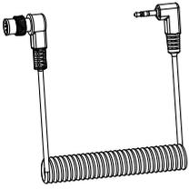
**DSLR Shutter Control Cable** - To connect the **DSLR Shutter Control Port** of **Star Adventurer 2i** to your DSLR's external shutter control port. This allows **Star Adventurer 2i** to directly control the DSLR's shutter release with preprogrammed shutter interval. You can order an optional cable for your camera from your local resellers. The Following list shows the cables that we offer as optional items.
