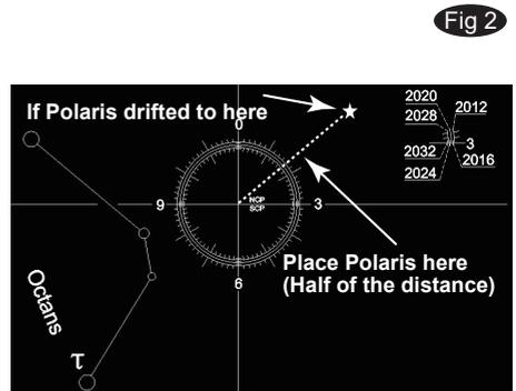
5. Repeat steps 1 to 4 a few times until the object remains at the center of the reticle when rotating the mount in R.A. axis.
