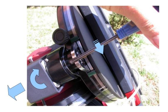
Installing the drive head is the reverse of removal. The retaining screws must face outwards and positioned symmetrically respect to the spring clip opening.
