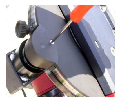
Using a 2mm hex key remove the 2 retaining screws (M2,5x5). Apply a drop of Loctite 243 when assembling the unit.
