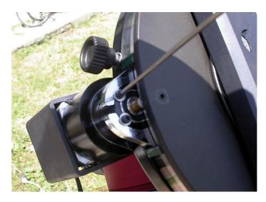
Using a 4mm hex key force the spring clips out and at the same time, grab the motor cover, twist and pull it in small steps until it is free from the clips.
