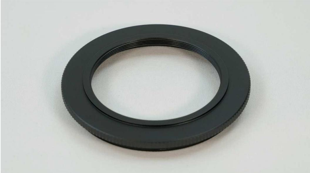
This dedicated camera adapter is designed for the FSQ-80FC optical tube assembly. When installed, it provides an M54 rear thread with a back focus of 56.2 mm, enabling compatibility with Wide T-Mount DX-WR adapters.
