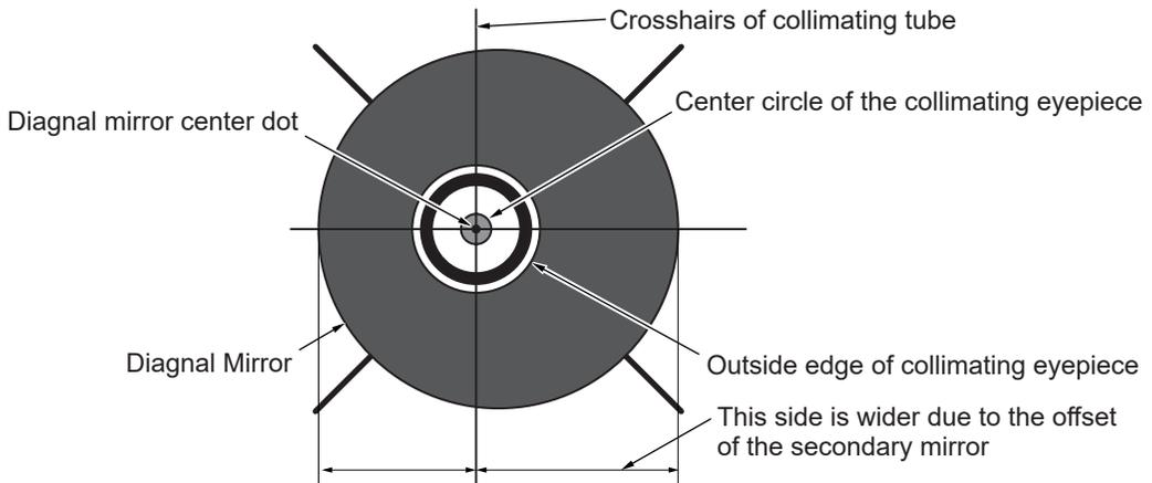
[ This figure illustrates the collimation of the correct secondary mirror. ]
