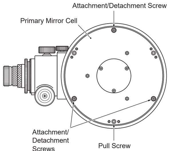
When attaching or detaching the primary mirror cell, be sure to use the attached primary mirror cell attachment/detachment screw.
