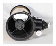
With an f/3.3 system the speed necessitates a large secondary that will illuminate the image properly. Placing the diagonal mirror in the center of the tube will produce uneven illumination across the field imaged. In order to fully illuminate the image circle the secondary must be offset to accept the full light cone produced by the primary mirror. The spider was specially strengthened to hold the mirror offset securely without any flexure.
