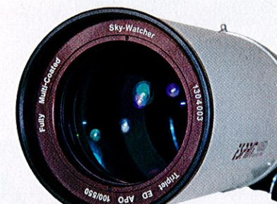
The f/5.5 objective elements are flawlessly multicoated, and the tube has one knife-edge baffle halfway down the tube to eliminate off-axis glare. The focal length as tested was 550 mm (21.7 inches) — just as advertised.
