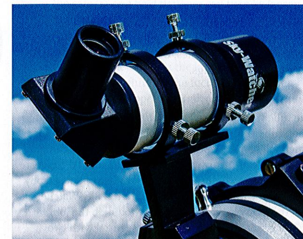
The included 9x50 finderscope is an erect-image, right-angle design. You can focus it by loosening the retaining ring at the front end and then turning the objective.
