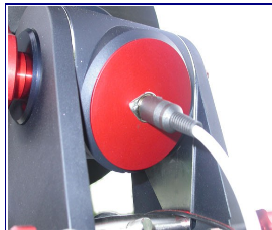
DEC and RA encoder connectors
