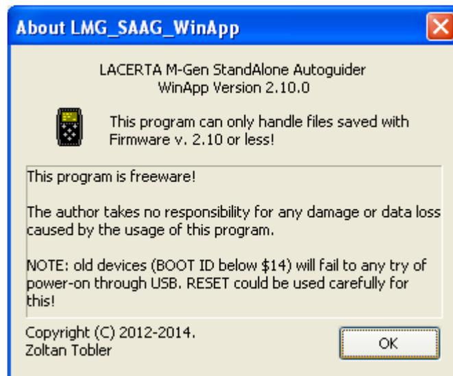
The PC application’s version show that highest verison number of the Firmware in the device that it can handle. There is always a new PC application for each new Firmware release. The users are advised to use the PC app. version equal to the running firmware to avoid some incompatible behaviour.
