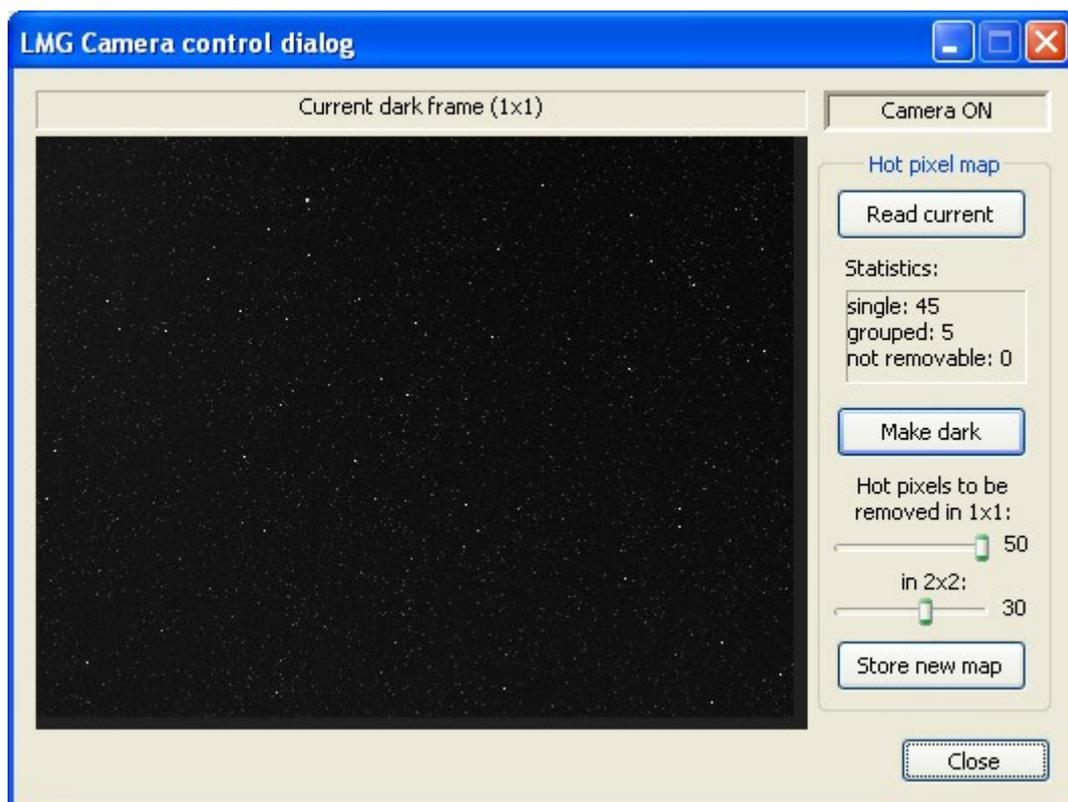
The displayed image is reduced in size by a factor of two, so each pixel shows the maximum of a 2×2 pixel block of the CCD. That's why You can see a lot of gray (“warm”) pixels besides the hots. Maximum must be shown to see every single hot pixel left (not cosmetized yet).
