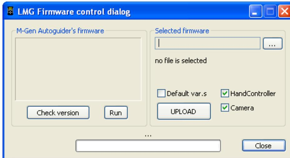
On the left box information or error is displayed about the autoguiders's current firmware. On the right, You can select a local firmware file (on Your PC) and get it uploaded into the autoguiders.
