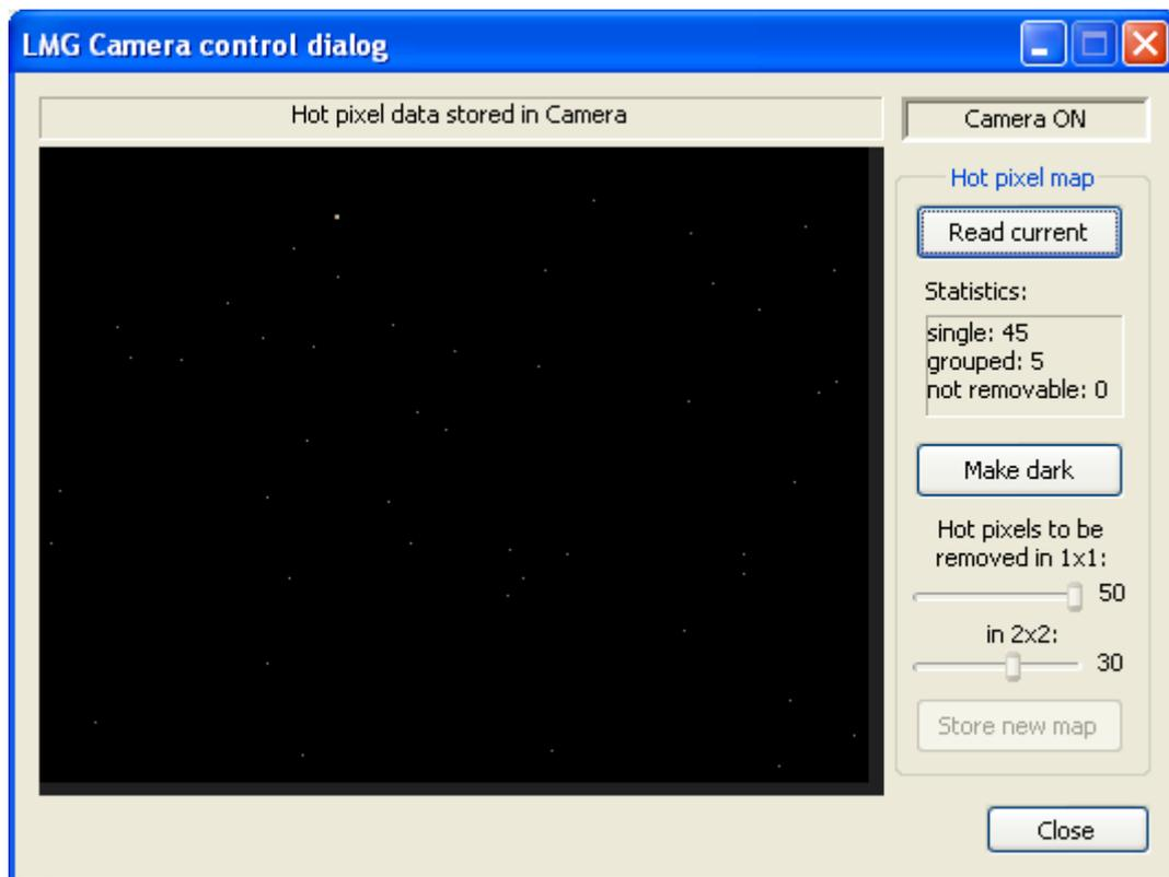
“Statistics” gives some info about the amount of different hot pixel types. Single hot pixels are surrounded with normal (non-hot) pixels. A grouped hot pixel is such that it has at least one neighbouring hot pixel. These could be cosmetized as well but with less efficiency, since there are less surrounding good pixel information. Not removable hot pixels are totally surrounded by another hot pixels, these are very rare and won’t be cosmetized at taking frames.
